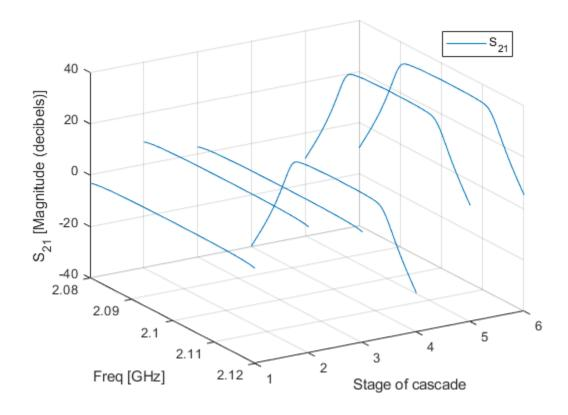
Plot the magnitude of the S21 parameter for the cascade at stage 6.
