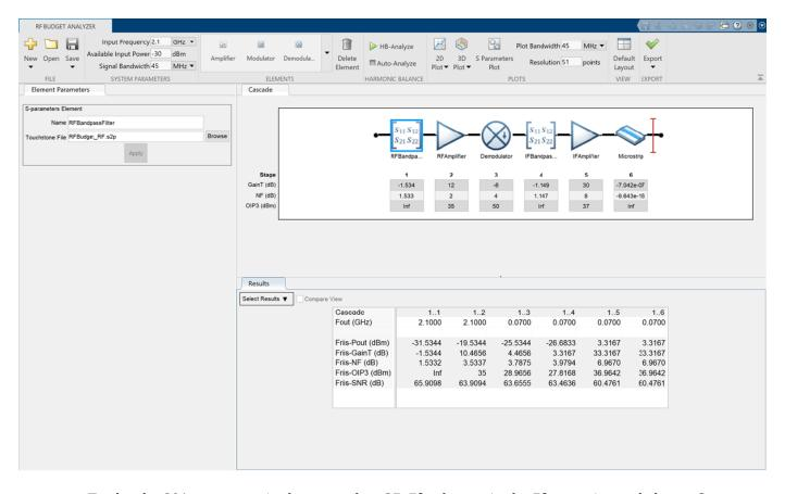
To plot the S21 parameter in the app, select **3D Plot** button in the **Plot** section and choose S-Parameters and then S21.
